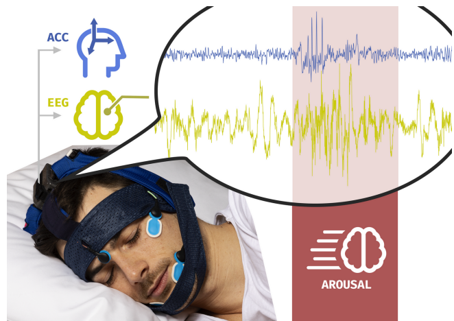
Fig. 1. The objective of this work was to use signals from a head-mounted accelerometer (ACC, blue) to detect sleep arousals and benchmark the real-time performance against the detection from electroencephalography (EEG, yellow) and expert reference labels (red shaded box).
