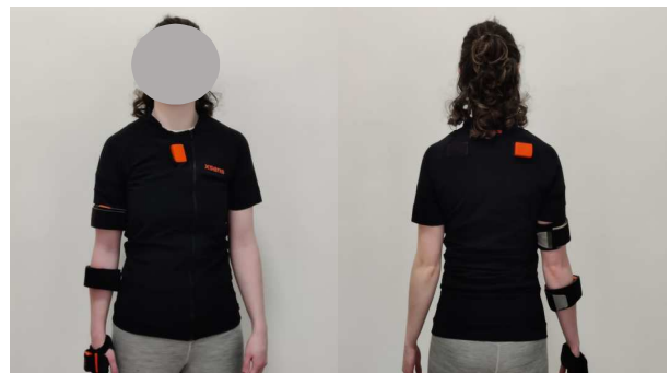
Figure 1. IMU placement on the shoulder, upper arm, forearm, hand and torso.
