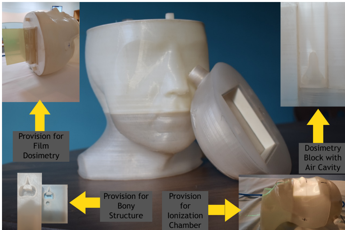
In-house 3D-printed anthropomorphic head and neck phantom with provisions for Ionization chamber and Films
